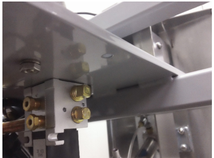
Fig. 7: Solenoid and chassis without air hoses attached
