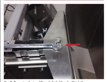
Fig. 8: Removing the two 10mm bolts holding the Weigh Hopper
