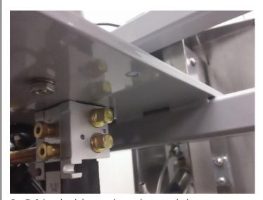
Fig. 7: Solenoid and chassis without air hoses attached
