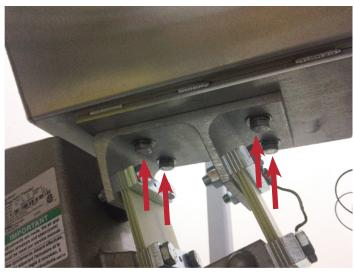
Fig. 3: (4) 5/16-18 bolts hold the Feed Pan to the Vibrator.
