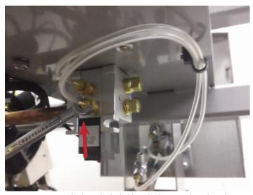
Fig. 6: Unscrewing the brass barbs holding the hoses to the solenoid
