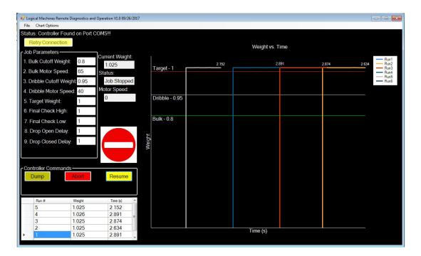
The user can also choose to overlay all runs in time on the chart. This may be an interesting way to visualize data if the user is looking to determine product weighing repeatability. Note: The user must clear all data from the table and chart before changing the chart options (Go to File > Clear Chart/Table Data).
